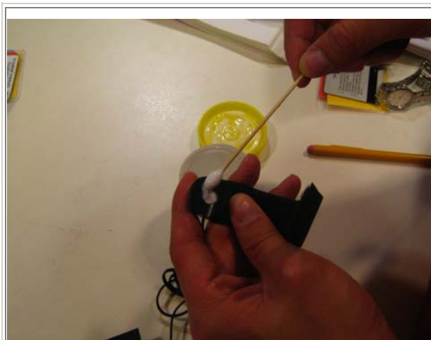
Image 24: Biopac gel being placed into the well of the electrode
