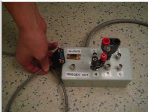
Image 4: DB-9 cable plugging into the BNC breakout box inside the scanner
