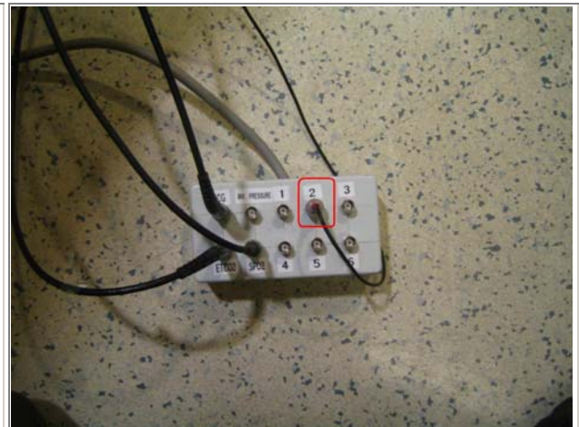
Image 9c: Banana plug plugged into the breakout box in the control room (note: plugged into channel 2 both in the control room and the scanner)
